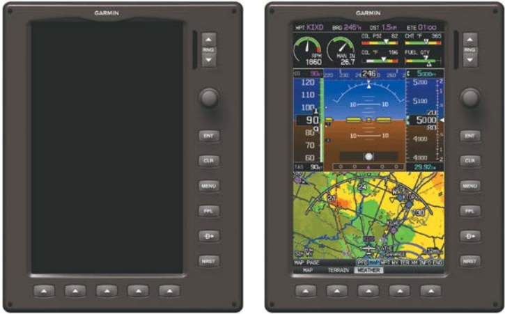
G3X Full-Screen Reversionary Mode (Failed PFD)
