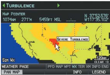
Severe Turbulence Selected With Map Pointer (Split-Screen)
