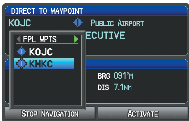
Direct-to Window (Flight Plan Waypoints Selected) (Split-Screen)
