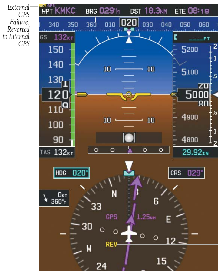
External GPS Navigation Failure
