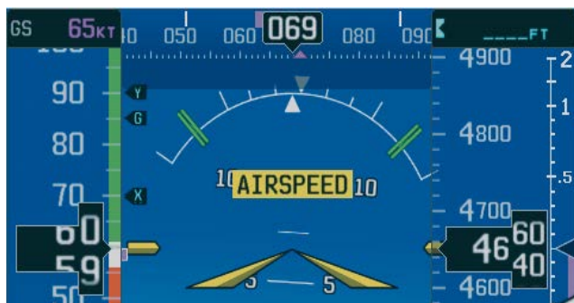
ESP Engaged (Low Airspeed)
