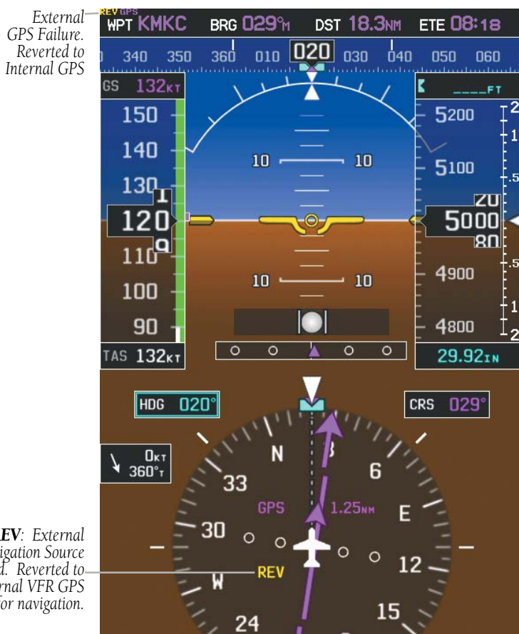
External GPS Navigation Failure
