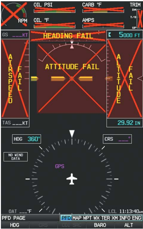
G3X System Failure Annunciations (Split-Screen)
