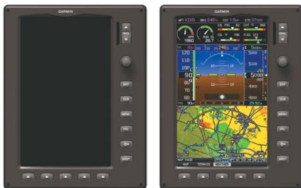
G3X Full-Screen Reversionary Mode (Failed PFD)
