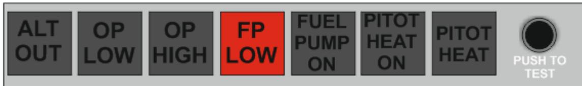
If the fuel pressure indicator falls below 2.2 psi / **FP LOW** warning is **ON**:
