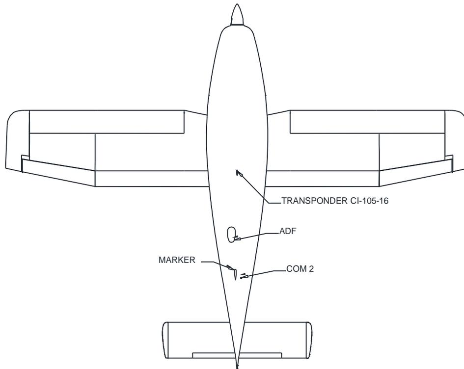
**Fig. 3. – Bottom view of antennas positioning on P2008 JC**
