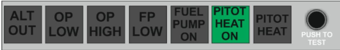
If the amber **PITOT HEAT** is turned ON, but the caution remains **ON**, the Pitot Heat system is not functioning properly.
