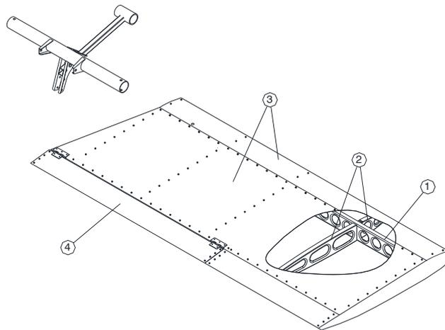
Fig. 7-2.STABILATOR STRUCTURE
